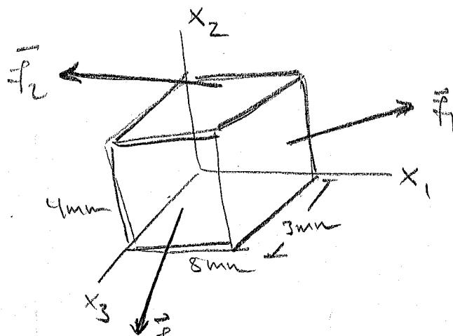
$$\bar{t}(\hat{e}_3) = \frac{\bar{f}_3}{(4\text{mm})(5\text{mm})}$$
