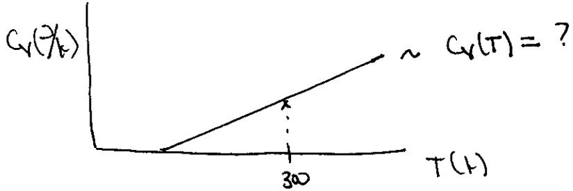
$$C_V(300\text{K}) = 7.5 \text{ J/K} \quad \Rightarrow \quad C_V(T) = 7.5 + \frac{2.5}{100} (T - 300)$$
