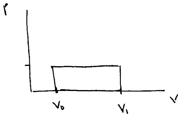
$$\bar{W} = p(V_1 - V_0)$$
